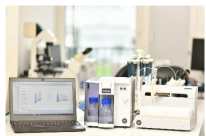
The Ampha Z32 Impedance Flow Cytometer set up in the Lab with the autosampler and a laptop showing measurement results.
