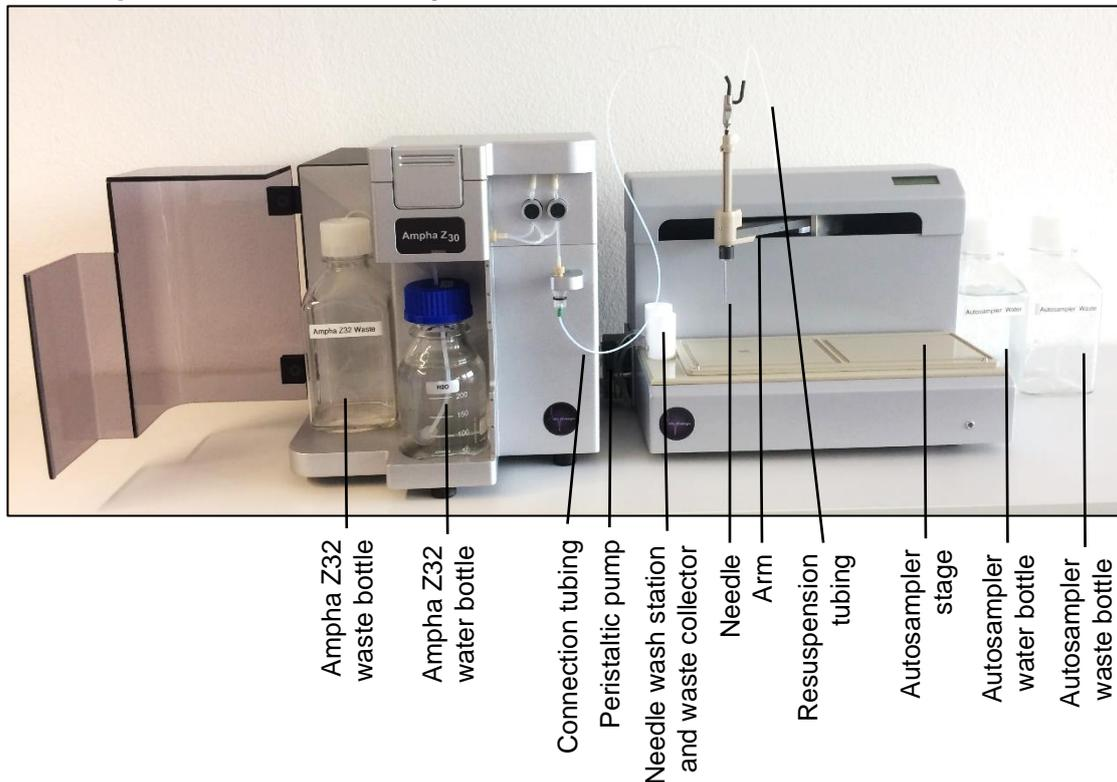
The autosampler features a sample resuspension functionality. After submerging the aspiration needle in the sample solution, air bubbles are released from the needle tip while the needle performs a linear bidirectional movement. This leads to the resuspension of sedimented pollen in the well. After resuspending, the sample is aspirated and loaded into the chip for measurement.
