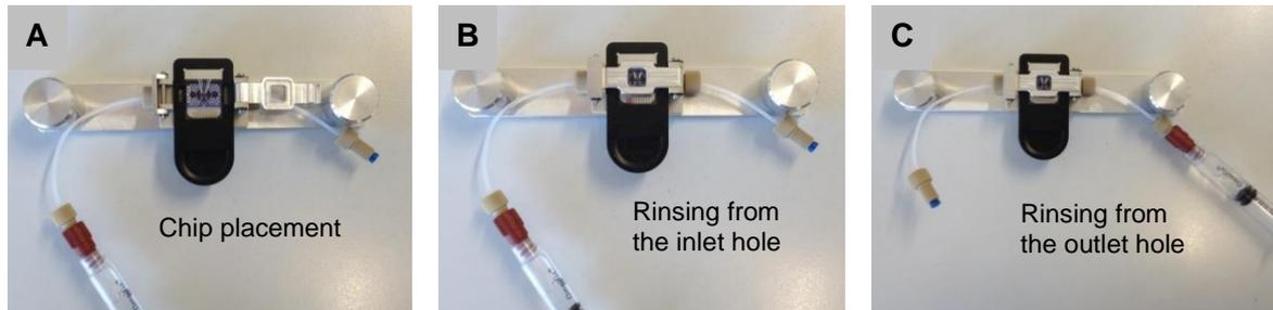
Cleaning should be started with  $< 0.5 \mu\text{m}$  filtered high-purity water. If necessary, other detergents can be used (table). Don't rinse with any organic liquids like alcohols.
