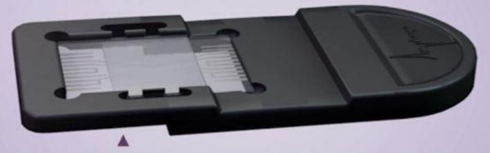
In this chip we measure changes of the electrical impedance of a fluidic medium when cells pass through the applied electric field.
