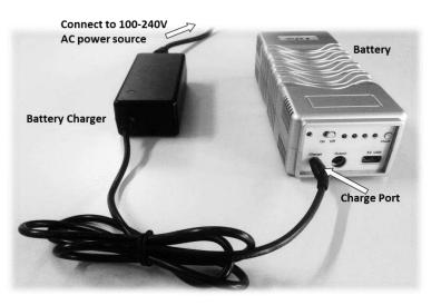
The bundled AC charger has dual-color LED lights to indicate the battery charging status: Red color = battery charging; green color = battery fully charged
