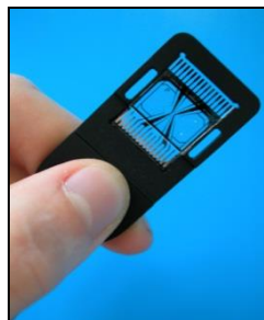
Fig. 2 Impedance micro-fluidic chip in holder frame.
