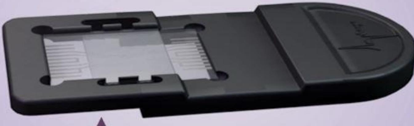
In this chip we measure changes of the electrical impedance of a fluidic medium when cells pass through the applied electric field.
